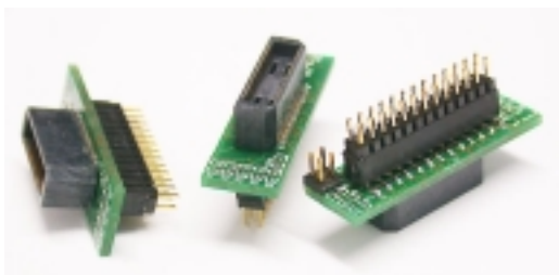
6. ITP700 (26 pin) – XDP (60 pin) adapter
