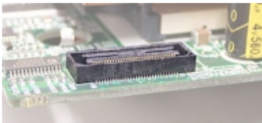
5. 60-pin male debug port header (XDP)
