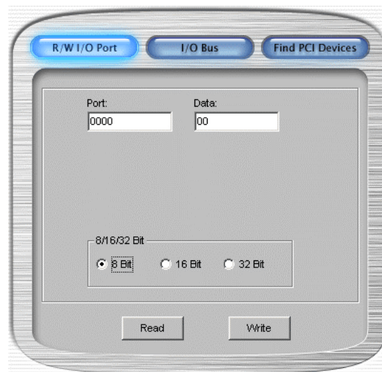
Fig. 8 – I/O port and Bus tests in Interactive mode
