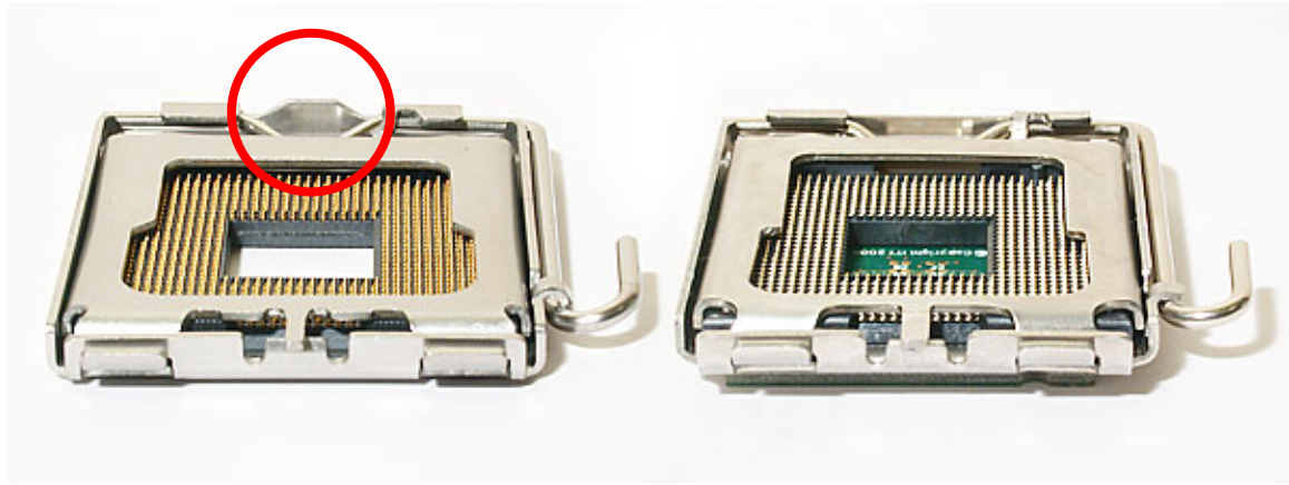
Figure 1.02 Tyco sockets (left) have a raised metal tab to limit the travel of the Load Lever – Foxconn sockets don't (right)
