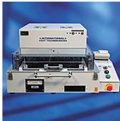
Fig. 2 – Fixture for Automated Connection
